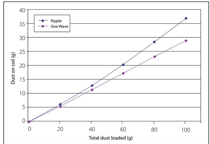
Figure 5. Effect of Fin Pattern on Dust Accumulation
