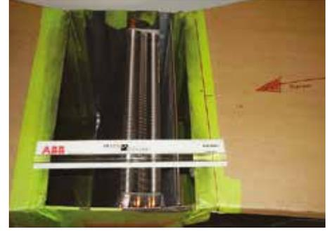
Figure 3. Dust Accumulation Test Setup
