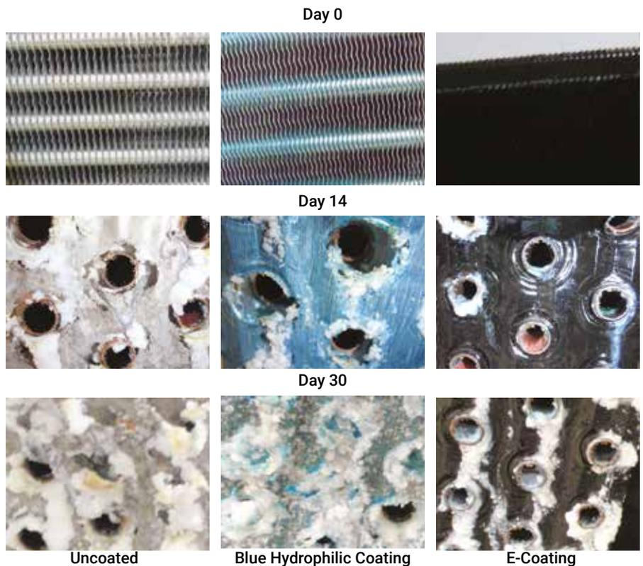
Figure 2. Salt Spray Test Samples and Results
